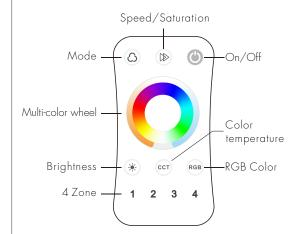
R8-5 can also be used as four zone universal remote, each zone can match single color, dual color(WW/CW), RGB, RGBW or RGB+WW/CW controller.
