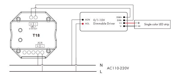
Note: We recommend the number of LED drivers connected to 0/1-10V dimmer does not exceed 100 pieces, the maximum length of the wires from dimmer to LED driver should be no more than 50 meters.
